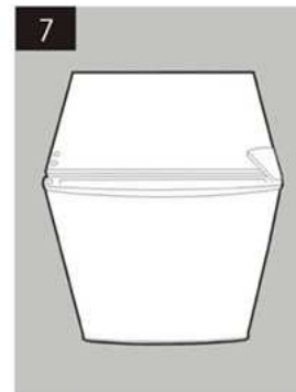
Check that the door is aligned horizontally and vertically and that the seals are closed on all sides before finally tightening the bottom hinge.
