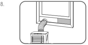
Insert the window slider adaptor into the hole of the window slider.
